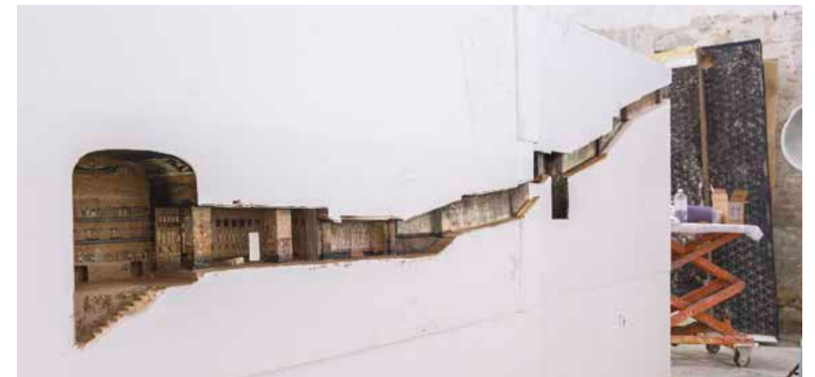
The Model of the tomb of Seti I made from 3D data recorded with the Faro Lidar Scanner and printed on an assortment of 3D printers.
