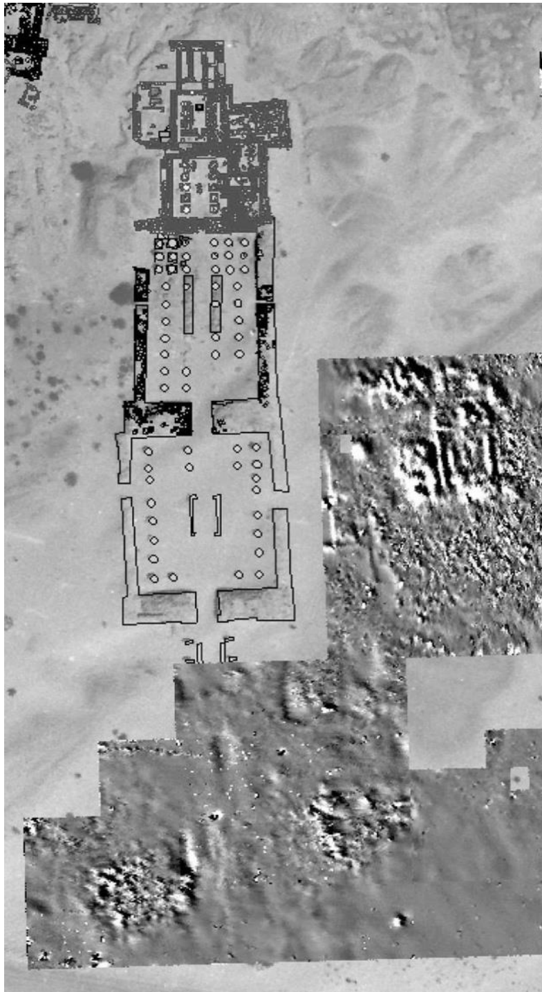
Fig. 77. Magnetic survey image generated in 2006 showing B 500 with previously unknown buried structures not visible from the surface: at right (NE): B 1700; below right: the mammisi temple and kiosk (B 560-561) and opposite that: a still unexcavated temple (B 570). (Geophysics: Meg Watters, T. Goldman, R. Wutzler, Pawel Wolf and Moh. Abdul Wahab.)
